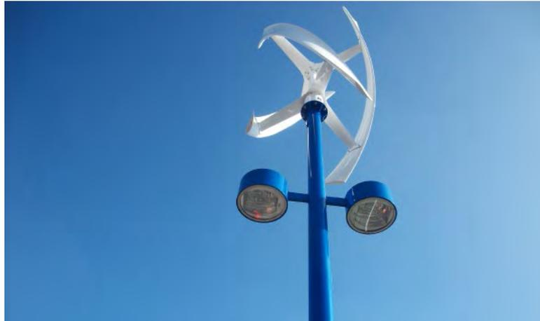
In November 2011, an **eddyGT wind turbine system** manufactured by Urban Green Energy was installed at Brighton Car Wash & Detail Center by Sullivan Energy Group in a monopole tower installation.
