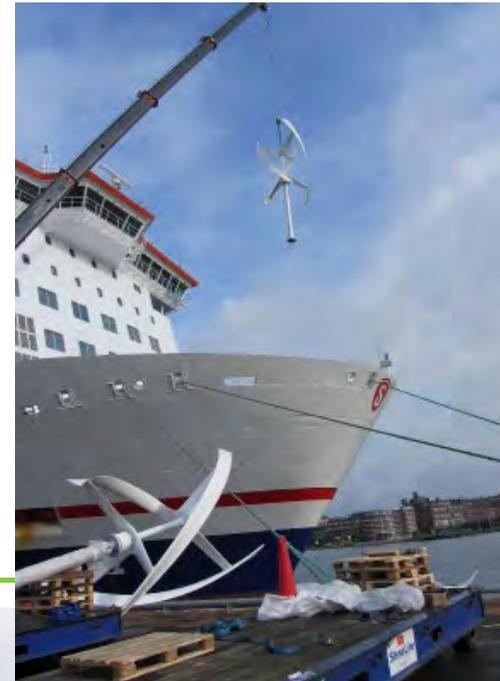
to use the aerodynamics of the wind leaving the turbine to improve the boat's overall aerodynamics. (CFD simulation showed the coefficient of drag decreased from 0.56 to 0.51 with the turbines installed.) The power generated by the turbines is expected to save on fuel as well as supplement onboard power systems, significantly reducing the energy costs of the boat when it is docked and minimizing its environmental impact.
